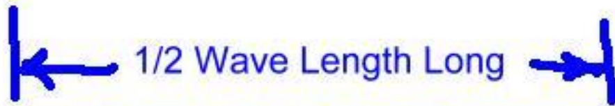
Simple Dipole Antenna
